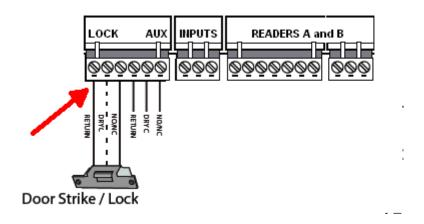
2. Use the following figure to wire the door strike/mag lock according to the power supply used. Be sure to use the S4 suppressor kits as shown below.
